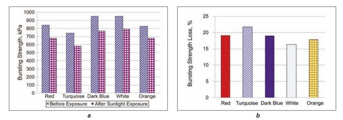
Fig. 5. Bursting Strength Results Before and After Sunlight Exposure (a); Bursting Strength Loss After Sunlight Exposure (b)
