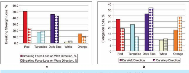
Fig. 4. Breaking Strength Loss and Elongation Loss of the Fabrics
